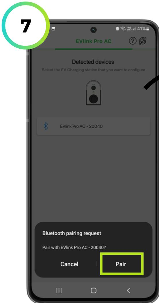
7. When prompted, allow your device to pair with the charge point. The LED on the charge point should blink several times to indicate that a successful connection has been established.
