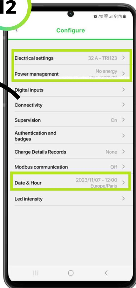
12. Return to the **Configure** menu and use the relevant sections to alter the **date/time** and **electrical settings** to meet the installation requirements.
