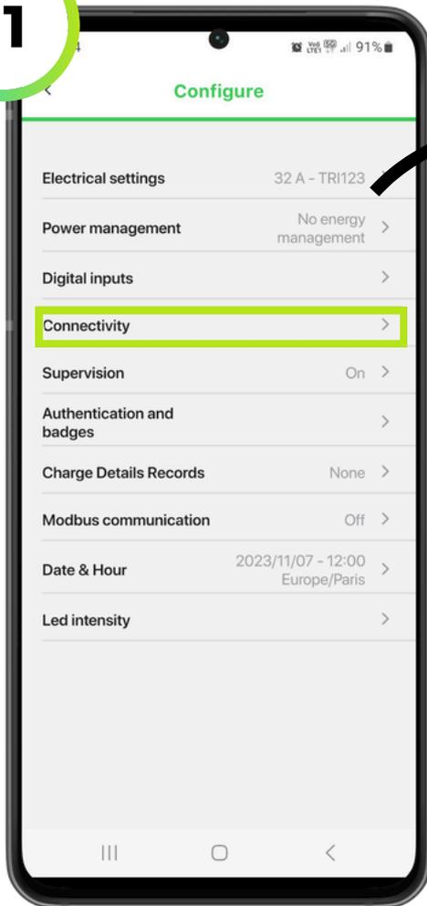
11. Select **Connectivity** to establish a network connection using the appropriate credentials.
