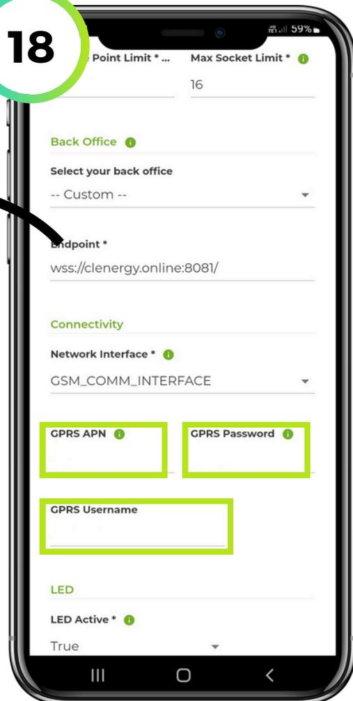
18. If connecting using a 4G/SIM network, enter **eapn1.net** in the GPRS APN field and **clenergy** in the GPRS password and **GRPS Username** fields.
