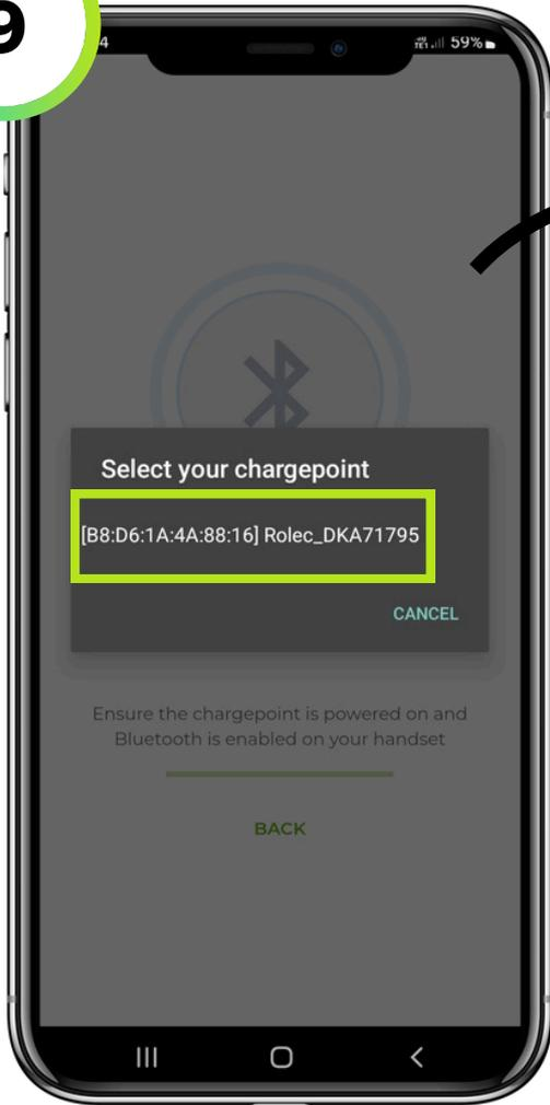
9. Select the relevant charge point from the list as identified by the serial number (more than one charge point may be displayed depending on your installation). Enter the password as located in the charge point documentation if prompted.
