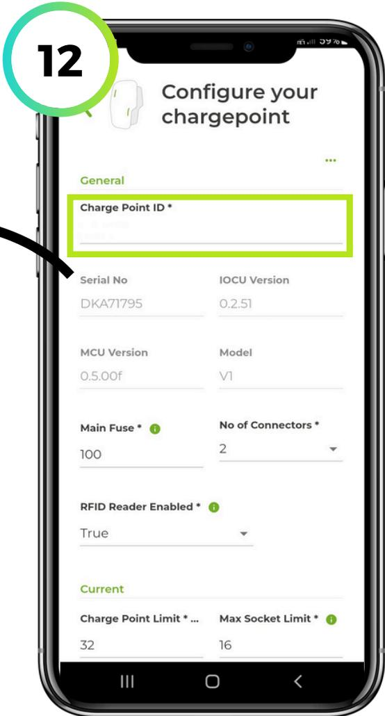
12. Enter the charge point serial number (as displayed with the product documentation) into the Charge Point ID field.
