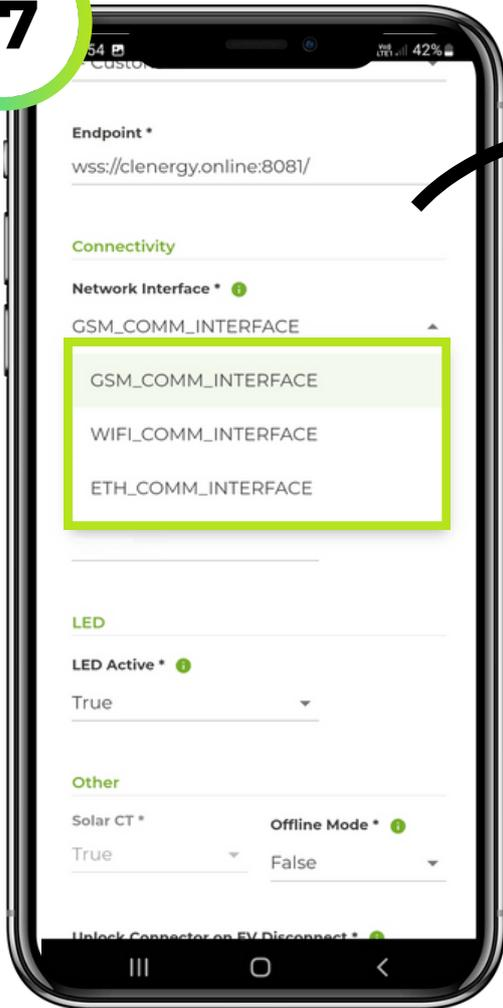
17. Select the relevant **network option** from the drop-down menu for your installation and enter the **required network credentials** to establish a connection.
