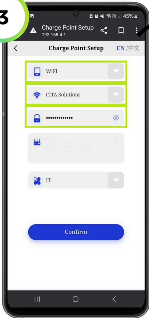
3. Select the correct network for your installation and join by entering the appropriate credentials in the 3rd field.
